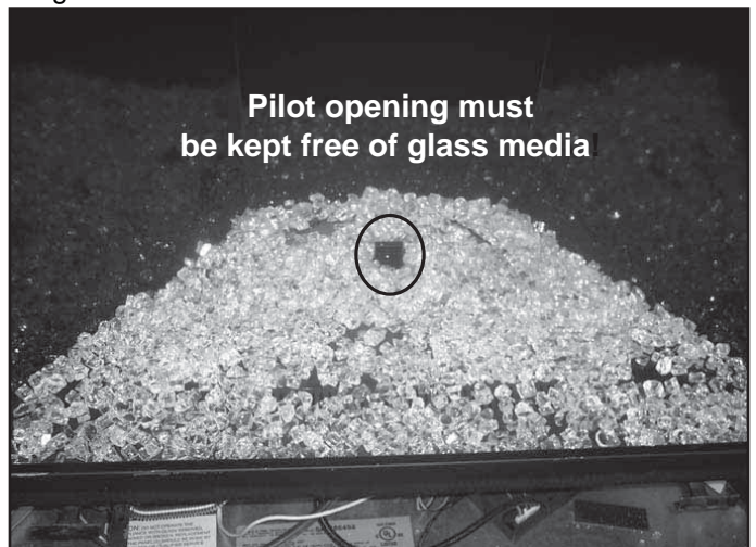
Figure 15.6 Pilot Open & Glass-Media-Free
